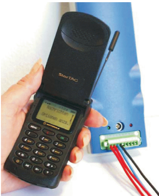
Controlling rectifier stations by mobile phone
